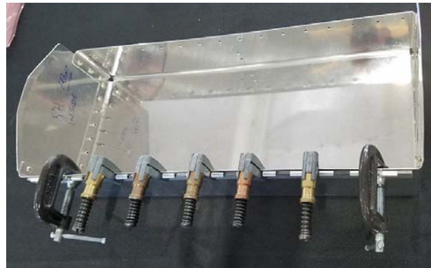
Use a ruler to accurately center the hinge.
