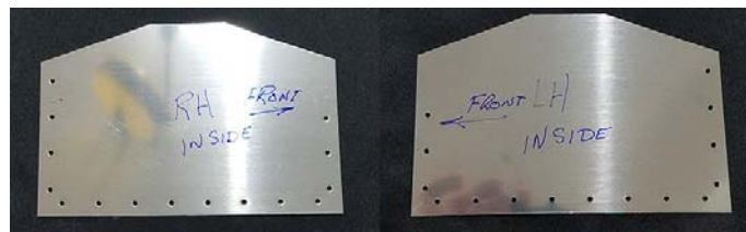
Help protect from making a mistake by clearly labeling orientation of the end pieces. Use blue Sharpie. (Not black.)
