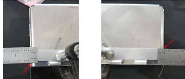
Use a ruler to accurately center the hinge.
