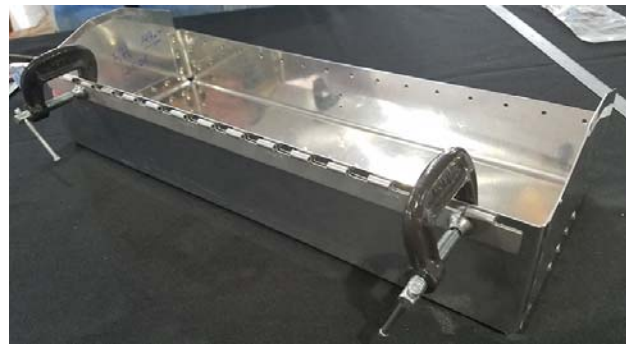
Loosely clamp the hinge in its approximate position.
