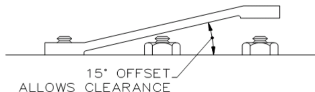
The 15-degree offset of a standard box end wrench can sometimes provide the clearance you need.
