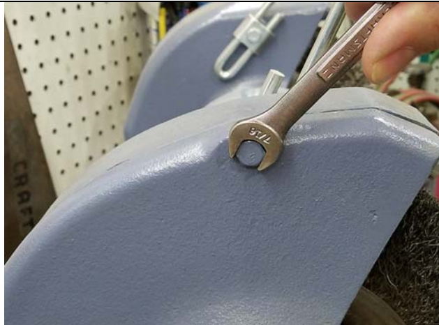
This bolt is completely accessible within the entire surrounding area that the wrench will be swinging.
